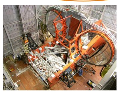
Two twin comounted 8.4 meter telescopes
