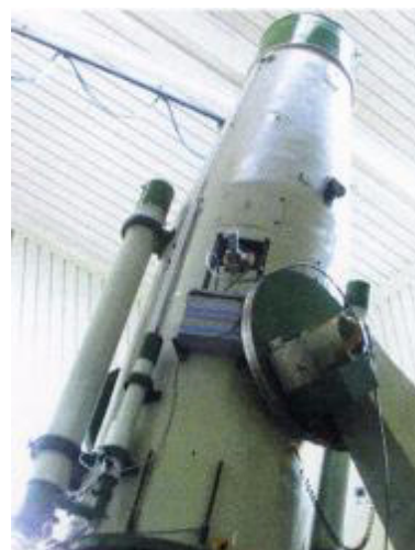
Figure 2 : The SCAM camera head and its electronics attached to the NW side of the S/67-92cm telescope at Cima Ekar
