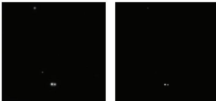
Fig. 3: Improvement of imaging by the lucky image technique: the binary Cepheid CE Cas ( left : without lucky imaging; right : with lucky imaging)
